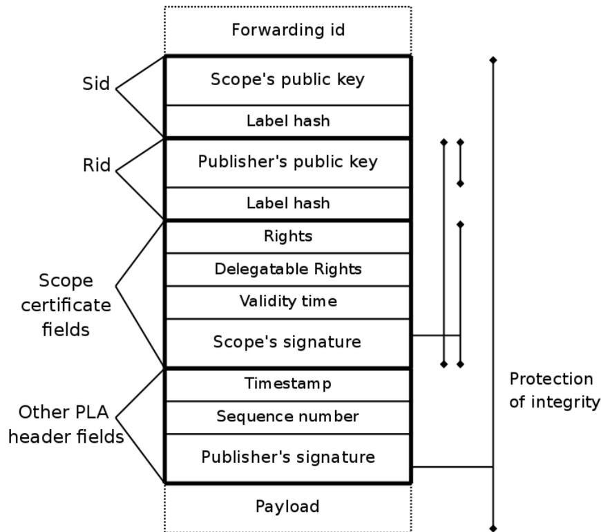
**Figure 4.10 – Overview of the packet header**
